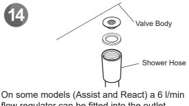
flow regulator can be fitted into the outlet. Note: Orientate flow regulator as shown
