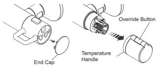
**5.** Remove the fixing screw holding on the handle attachment components using a 2.5 mm Allen key. Remove the two attachment components.
