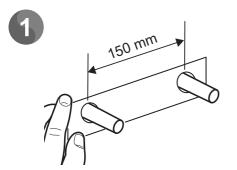
Fit the plastic pipe guide over the inlet pipes. Level the pipe guide and secure to the wall to hold in position. Leave the guide in place and finish the wall.
