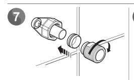
Install the olives and the connectors. Tighten finger tight and then another 1/4 to 1/2 turn.
